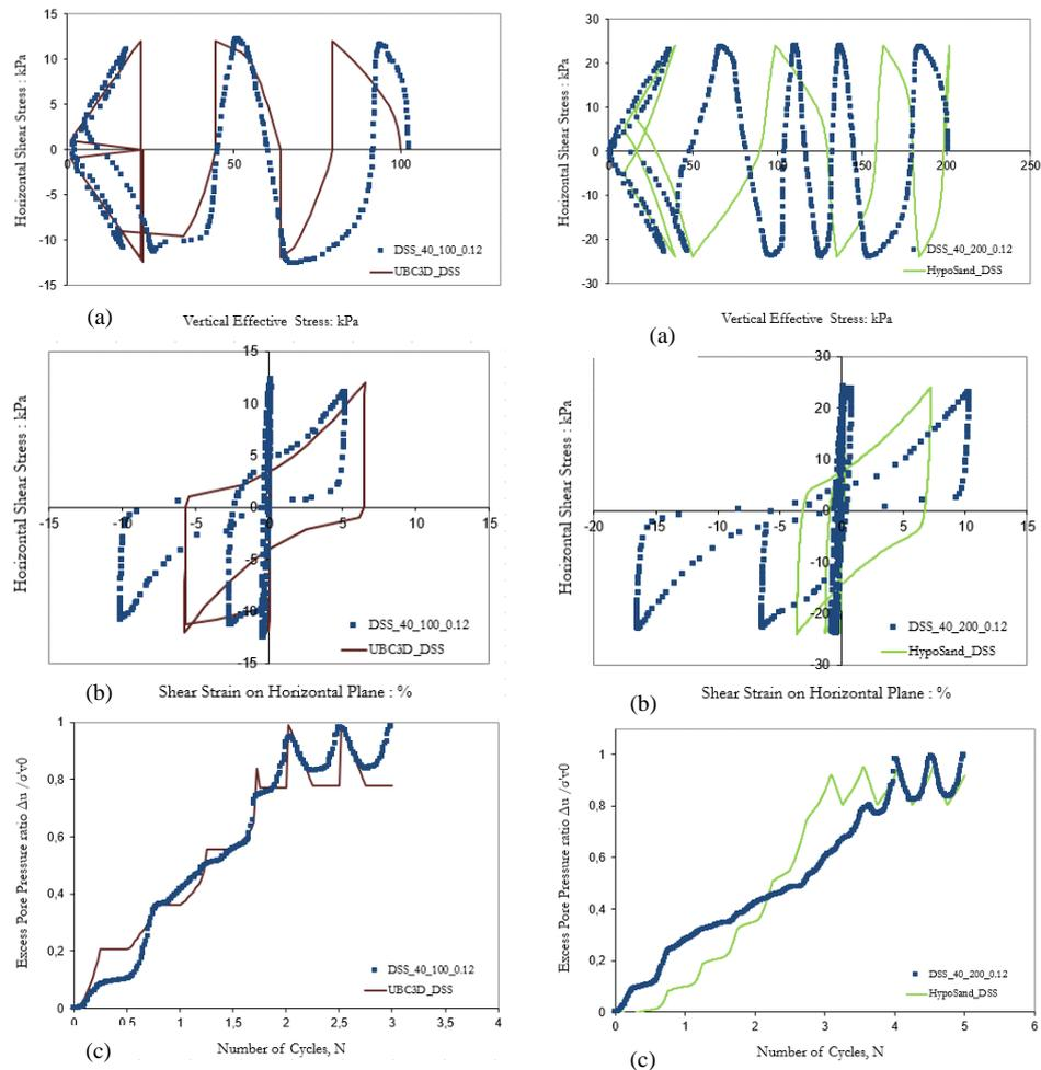
Figure 2. Test 1 (left) reproduced with UBC3D and test 2 (right) reproduced with Hypoplastic model.
