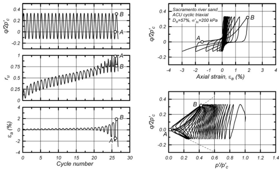
Figure 1. Medium dense sand under undrained conditions [1]
