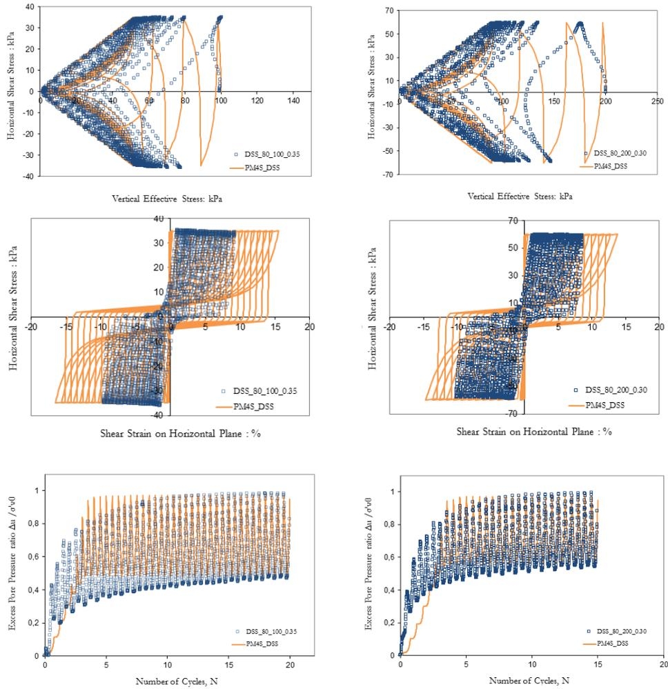
**Figure 3.** Test 3 (left) and test4 (right) reproduced with PM4Sand model.
